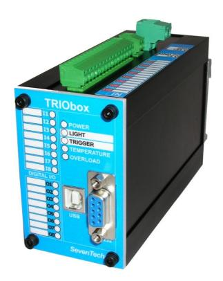
TRIObox compact device efficiently combines three components often used in machine vision.
